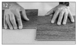
12. To disassemble the individual planks slide the short ends apart while the boards remain flat to release, lifting the short end at an angle will cause damage to the joints.
