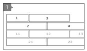
1. The flooring needs to be laid in a brick pattern, it may be necessary to cut the first board, the balance of this can be used later to finish a row.
