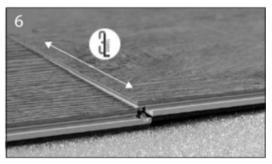
6. The short ends are lowered into position to lock the planks together
